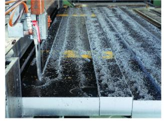
This special structural steel HYT 60® is most suitable for the construction of valves and hydraulic parts because of its excellent machinability on drilling and milling.
